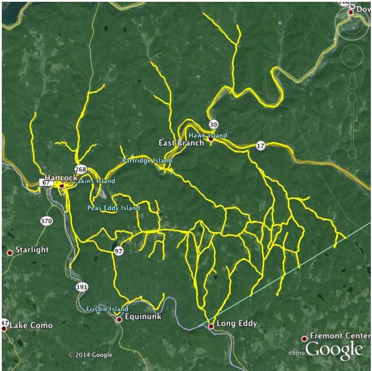
Figure 1. Ground Level Ambient Air Methane Survey of the Town of Hancock, Delaware County, New York. 15-16 September 2014. Yellow lines indicate roadways travelled and tracks of methane measurements during the survey.
